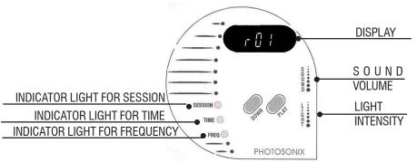
The 3 LED DISPLAY shows the session that is playing and also that session's parameters while it is playing. The single LEDs will light up to show which function value the 3 digit display is showing. For example:
